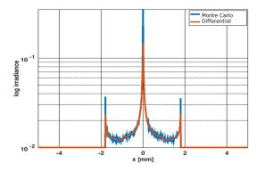
**Figure 1.** Ghost light distribution on a detector. Compared are the results of differential and conventional ray-tracing.
